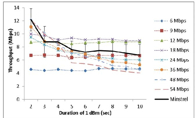
Figure 4. Throughput with rapid channel variation
